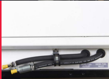
Input/Output fuel pipe
