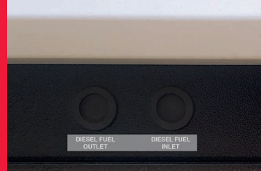
Input/Output fuel pipe
