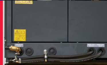
Input/Output fuel pipe
